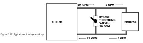
**b.** Some models may have a factory installed bypass. Adjust the valve accordingly.
