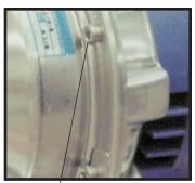
Typical pump casing bolt
