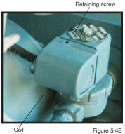
The plunger is "loose" inside the enclosing tube. Be certain it is retained in the enclosure tube as the bonnet is removed (figure 5.4C).
