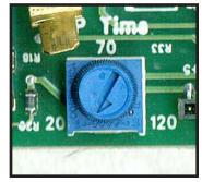
Low Pressure Potentiometer. Figure 3.3C
