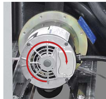
Correct shaft rotation is clockwise.
