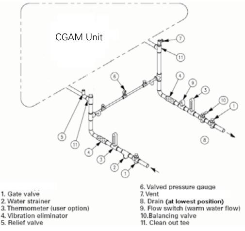
**Note:** In addition to those recommended for field piping, the CGAM unit includes factory installed manual air vent and water drain valve with partial heat recovery option. See Figure 81, p. 96 through Figure 83, p. 97 for partial heat recovery component locations.
