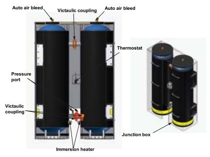
Figure 80. Buffer tank components - slant 20-35 ton & V 40-70 ton
