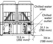
Water connections are 25 in (635 mm) from unit end.
