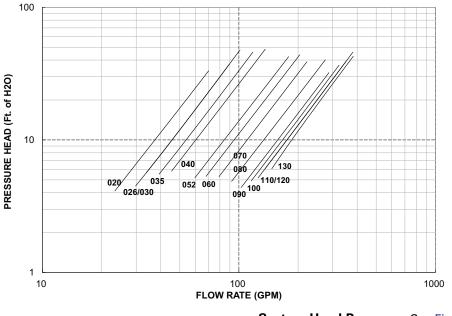
**System Head Pressure**. See Figure 66 for the system head pressure available.
