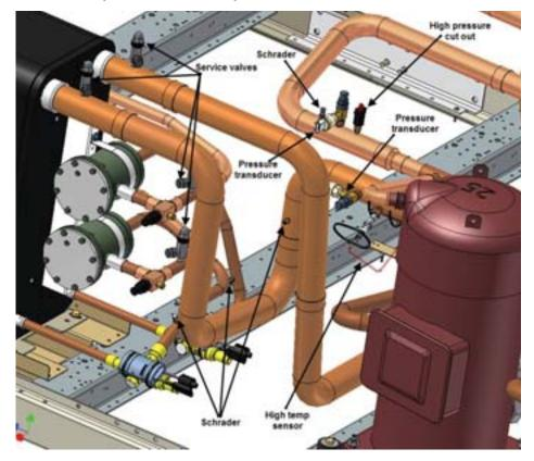
Figure 72. W 80-130 ton component location - evaporator side
