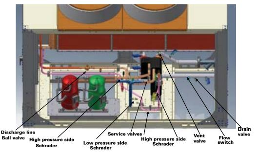
Figure 69. V 40-70 ton component location - circuit 1
