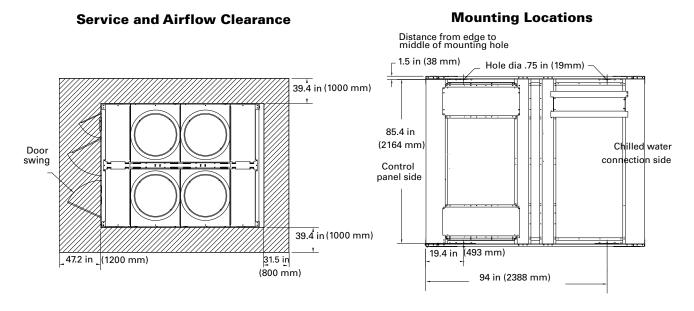
More clearance may be needed for airflow depending on the installation.
