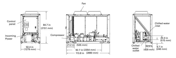
Water connections are 1.7 in (44 mm) from the end.
