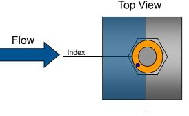
The flow switch must have the dot in the shaded area to the left of this line for proper indexing (±90° off Index)
