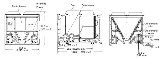
Water connections are even with unit end.
