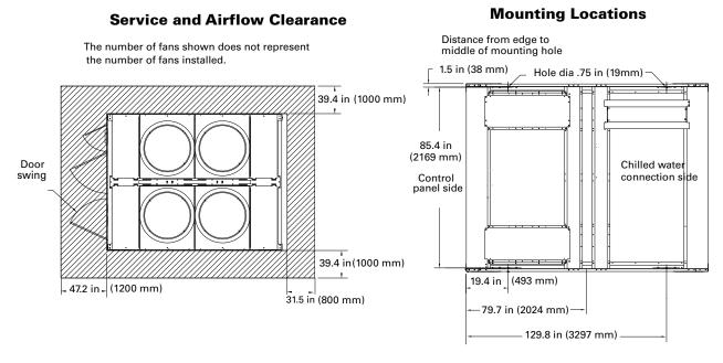
More clearance may be needed for airflow depending on the installation.
