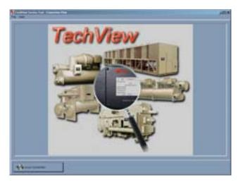
TechView is the PC (laptop) based tool used for servicing Tracer CH530. Technicians that make any chiller control modification or service any diagnostic with Tracer CH530 must use a laptop running the software application "TechView." TechView is a Trane application developed to minimize chiller downtime and aid the technicians understanding of chiller operation and service requirements.
