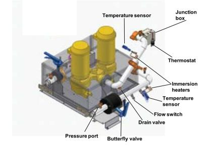
Figure 74. Pump package components, slant 20-35T, view 2
