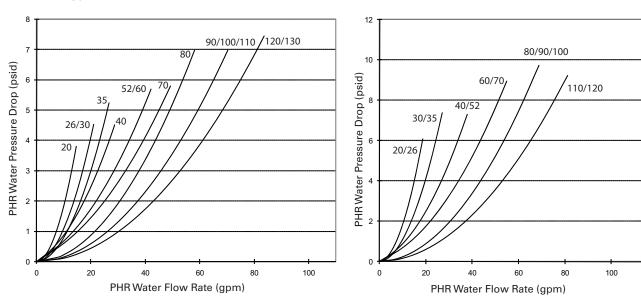
Figure 58. Partial heat recovery pressure drop curve -
