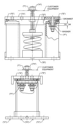
Figure 42. M2SS Seismic isolator installation reference
