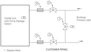
Field water piping pump package unit
