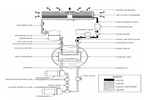
Diagram of Typical Air Cooled Chiller Refrigeration Cycle
