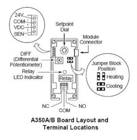
**Set Point Adjustment:** Set point is defined as the temperature at which the compressor will be shut off. Use the Set point Dial on the front of the temperature control to adjust the set point. The set point is factory calibrated at mid-scale to a tolerance of +/-1°F. Set point tolerance at the extreme ends of the set point range in relation to the printed scale may vary as much as +/-3°F
