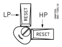
If the lockout is caused by the controls high side cut out, allow the pressure to drop at least 60 PSI below the cut out set point press and release the HP RESET button on the top of the control to restore operation of the chiller.
