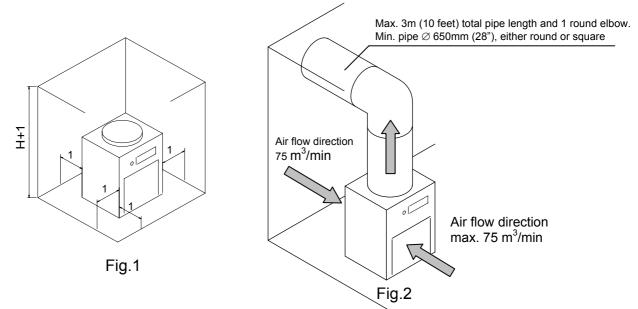
**Figure 1**: In case of installation in a small room it is imperative that the room has an appropriate ventilation system to evacuate all the heat generated by the chiller as explained before on this same point. If the heat is not removed the temperature in the room will quickly increase beyond the operating limits of the unit and it will stop by high pressure alarm (see point 3.1).
