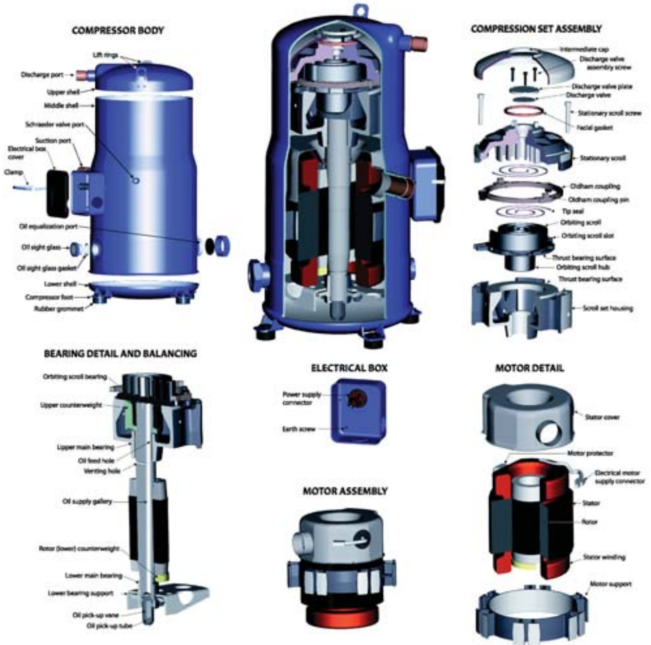
Figure 88. Compressor Internal Components, 15-30T
