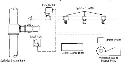
Water Flow Switch used as a safety control to activate alarms or signals, and to start or stop mechanically when fire occurs,
