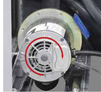
Correct shaft rotation is clockwise.
