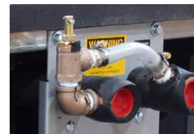
Typical optional automatic low flow bypass valve.
