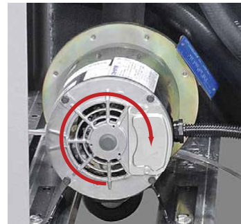
Correct shaft rotation is clockwise.
